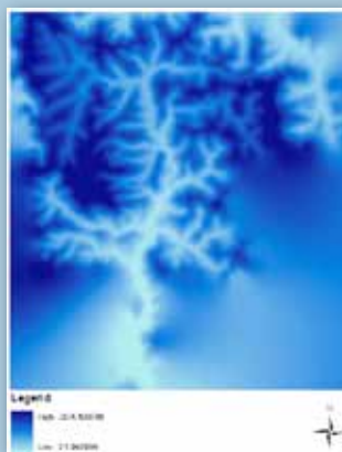
Figure 5: Contour layer in Raster format after Fill operation
